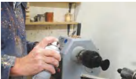
▲ Pic.9 After sanding down to 400 grit, cut back with synthetic fine wire wool. Give the hat a coat of sanding sealer followed by black lacquer
